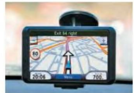
A GPS uses satellite signals to find your position in the earth's coordinate system with amazing accuracy.
